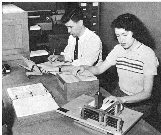
FIG. 5-40 National Bureau of Standards peek-a-boo punch and viewer in operation.
